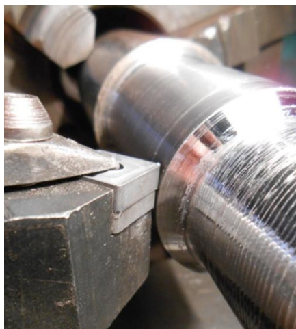
Figure 6 – Position of the cutting plate relative to the shaft in determining fracture resistance on lathe
