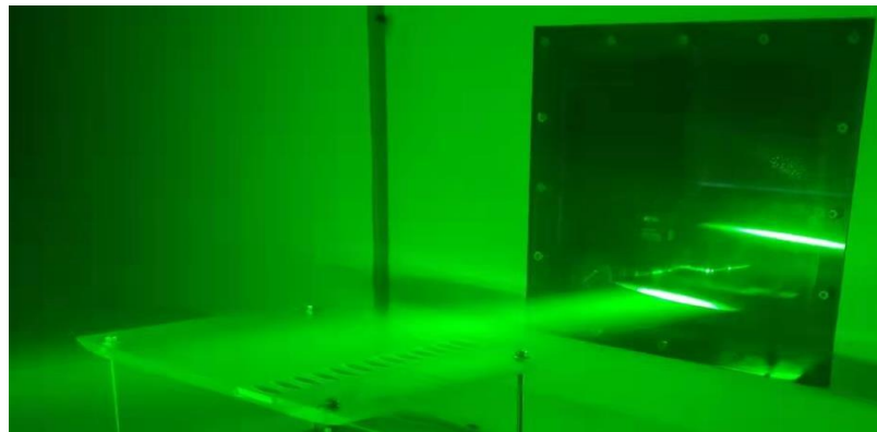
Fig. 4. A test model in the process of PIV measurement
