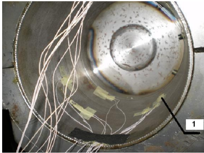
Fig. 2 Rope drum (location of measuring strain gauges)
