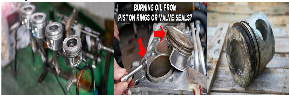
Figure 2. and 3. Oil leakage on the seals and Damage to the piston
