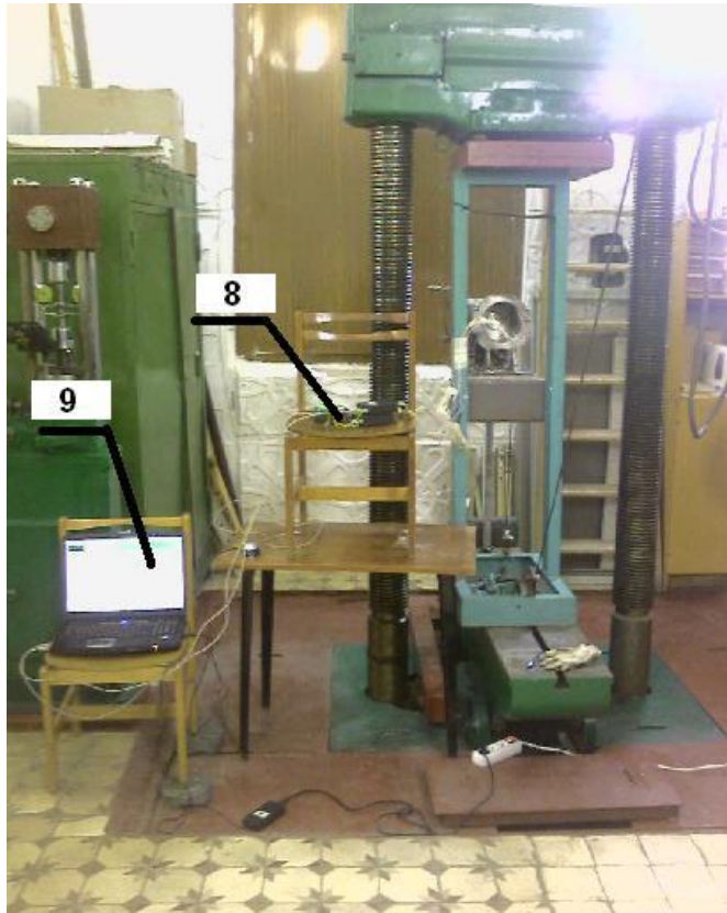
Fig.3 General view of the installation with voltage recorder ZET 210
