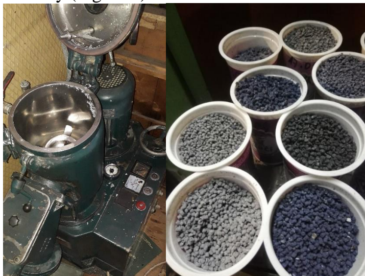
Figure 6. Hot mixer (10 L) for PVC melting and homogenization with plasticizers (left) and PVC re-granulates produced by injection molding (right)
