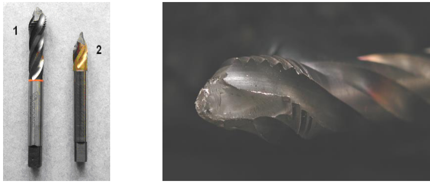
Fig. 2 The appearance of damaged cutters prior to thread cutting in the sleeve
